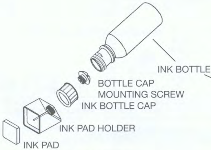
STANDARD INK RESERVOIR (Ink feeds with gravity assistance)
